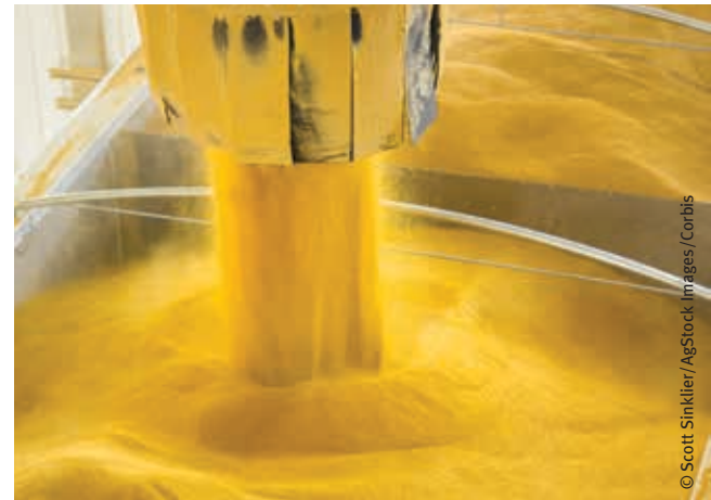
From left: Corn harvested and stored in silo. Ground corn being loaded into a grain truck after it has been used for ethanol production at Big River Resources ethanol production plant near Burlington, Iowa. This byproduct is known as distillers grain and will be used for commercial feed for cattle.
